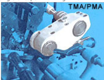
Thread Milling ATT.(25290000) Polygonal Milling ATT. (25296000) Max. length of thread: 22mm Max. pitch of thread: 2mm Max. speed of main spindle: 4,000rpm
