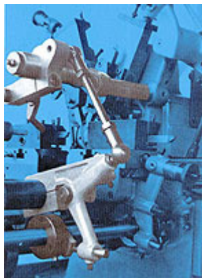
Overhead Swing Stop(25182000) Applied for some special set up when a standard stop is not applicable.
